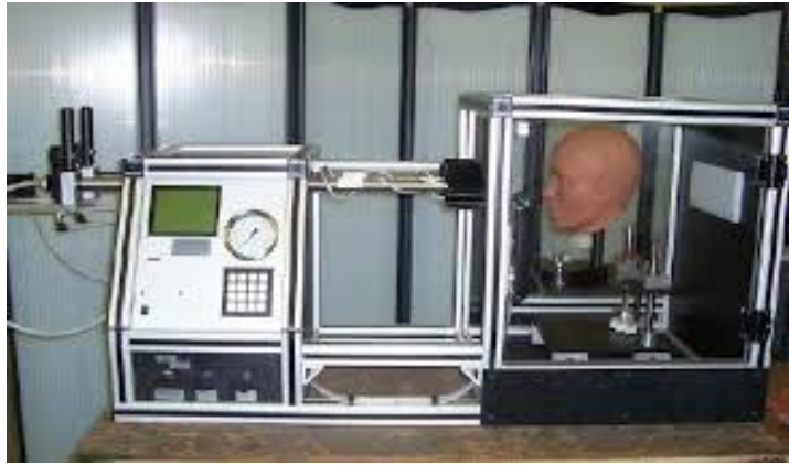
Figure E1 - High Velocity Impact Test Apparatus The unit shown above or its equivalent is suitable for the high velocity impact test
